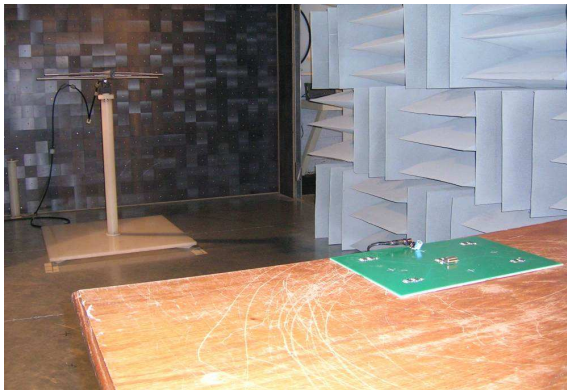
Figure 10: Emissions test set-up
